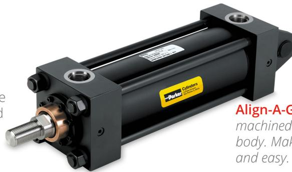
**Align-A-Groove** - A  $\frac{3}{16}$ " wide surface machined at each end of the cylinder body. Makes precise mounting quick and easy.
