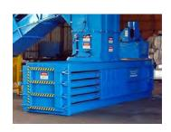
The HBM 4242 - 65C is an automatic cycling, short stroke baler with manual tie. This machine is fitted with cutting knives and is ideal for cardboard, and paper. The unit is activated when the hopper is full by a photocell.
