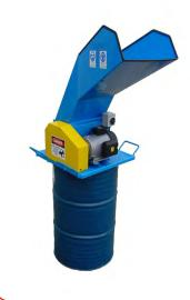
The bottle buster BB1200S is a versatile mobile unit that can be situated on top of a 205 litre drum or set up on rails over cullet bins or bays. The unit can easily be handled by two people, enabling it to be moved wherever needed. The wide hopper opening allows for easy dispensing of complete containers of bottles and glass jars for culleting.
