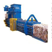
This machine is ideally suited for printers and small warehouses where automation is a prime consideration. The HBA 3040-50C is controlled by PLC for minimum operator intervention. With a capacities of up to 2.8 tonnes/ hour, this machine will solve your waste problems as well as reduce removal costs.
