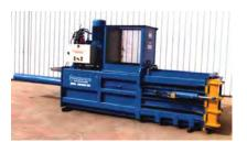
The HBM 3030-35C is an automatic baler with manual tie. This machine was specifically designed for baling plastic bottles such as PET, HDPE and PVC. The unit is activated by a photocell when the hopper is full.
